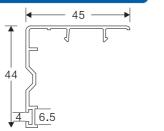
CASEMENT 12MM GLASS BEAD Code: SB-4002 WEIGHT(KG/M): 0.27
