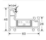
60 SINGLE GLAZING BEAD CASMENT Code: SB-4001 WEIGHT(KG/M): 0.317 LENGTH: 5.9 M
