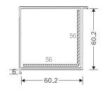
IN-LINE ADEPTOR Code: SB-2006 WEIGHT(KG/M): 0.307 LENGTH: 5.9 M
