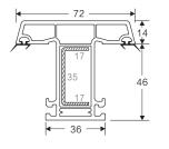
85 SLIDING DOOR SASH 2 Code: SB-1005 WEIGHT(KG/M): 1.22 LENGTH: 5.9 M
