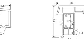
FRENCH MULLION / LAP JOINT Code: SB-3005 WEIGHT(KG/M): 1.067 LENGTH: 5.9 M
