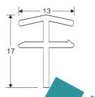
SHUTTER GLAZING BEAD Code: SB-SGB WEIGHT(KG/M): 0.26 LENGTH: 5.9 M
