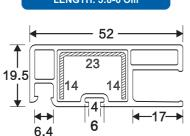
SLIDING 12 MM GLASS BEAD Code: SB-2001 WEIGHT(KG/M): 0.18 LENGTH: 5.9 M
