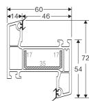
60 SMALL FRAME Code: SB-3007 WEIGHT(KG/M): 0.890 LENGTH: 5.9 M
