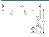
92 SLIDING DOOR SASH COVER Code: SB-2005 WEIGHT(KG/M): 0.227 LENGTH: 5.9 M
